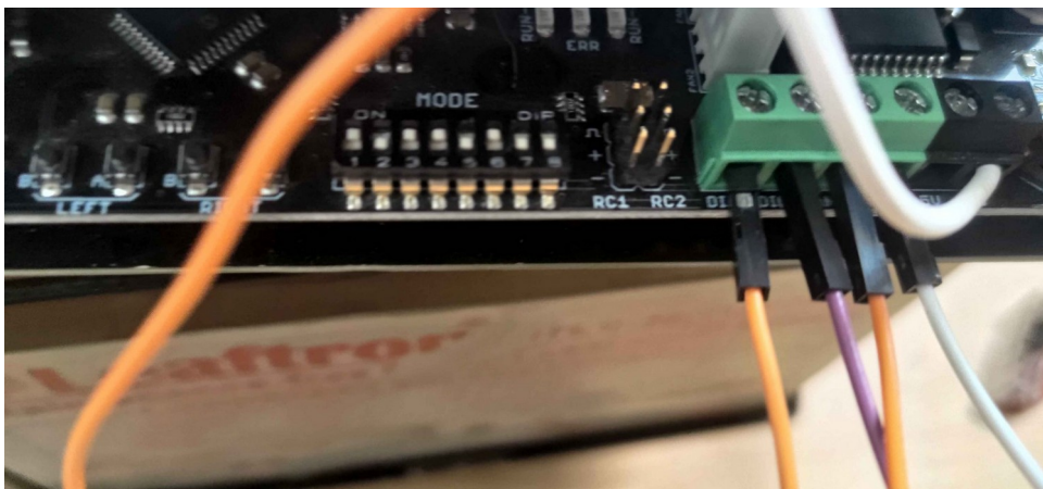
Figure 6. The MDDS60 DIP switches and the DIG1/DIG2/RC1/RC2 input row; this is where the incorrect AN1/AN2 connection forced the controller into single-channel mode.
