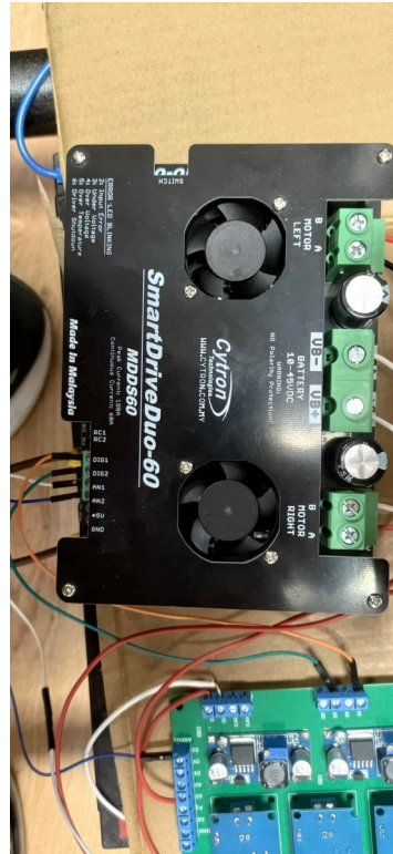
Figure 3. The Cytron SmartDriveDuo-60 (MDDS60) motor controller. The motor and battery connectors are on the right; the control inputs (RC1, RC2, DIG1, DIG2, AN1, AN2, +5V, GND) are on the left.
