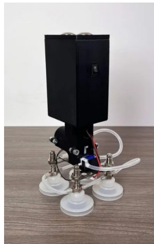
Figure 4. Vacuum gripper in operation
